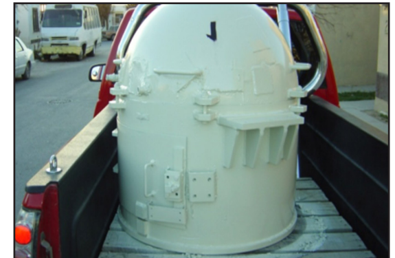
First mill after repair ready for delivery
