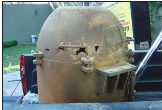
Worn mill after failure of rubber and fiberglass
