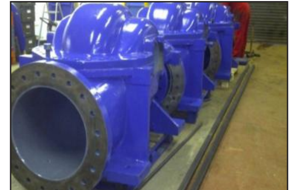
Coated pumps with ARC S2 inside and ARC S1PW outside with UV resistant top coat
