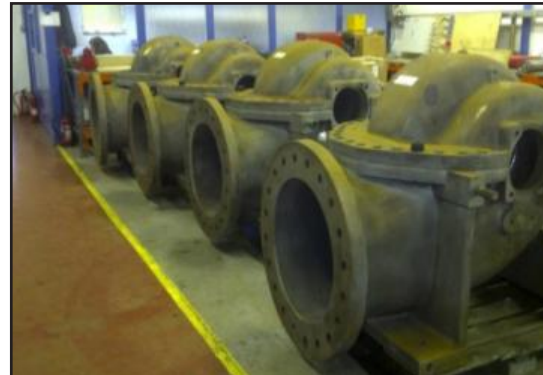
Pumps blasted and awaiting coating
