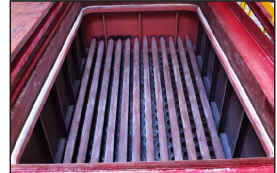
Bag house protected with ARC S7 in service over 2 years with no failures
