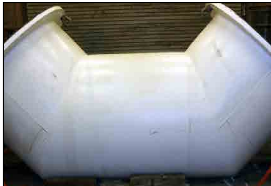
Exhaust elbow in shop laydown
