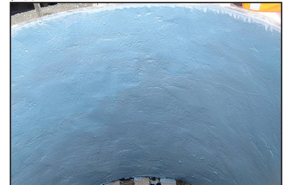
Chute protected with ARC BX1 over rubber and worn metal.
