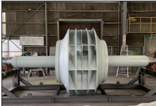
ID Fan in paint shop.
