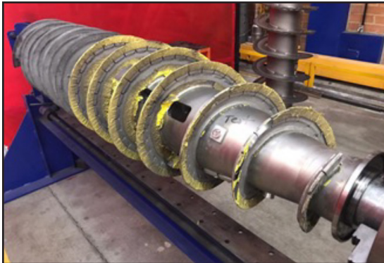
Screw with tungsten carbide inserts being welded in place.
